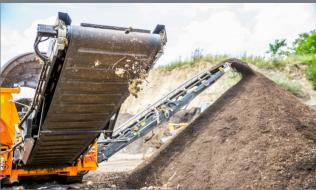
The SM 620 K Plus renders its services resting on a robust two-speed steel track chassis using 500mm wide steel tracks.
