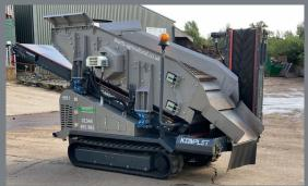
The KOMPATTO SC 221 tracked screening machine is the smallest self-propelled screening plant on the market today. Lightweight, compact-sized and featuring a robust chassis, it was designed for rubble and debris screening of material coming from construction and demolition, excavations waste, compost, asphalt, rock etc. It features a vibrating 2.2×1-mt double deck with, interchangeable screens and meshes to meet all needs, and it also includes three extracting belts.
